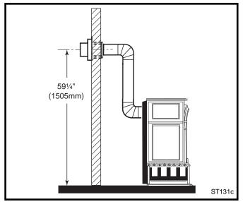
Fig. 20 Minimum wall thimble centerline.
